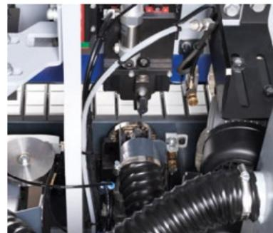
**Infrared heater for better edge adhesion on cold workpieces**
