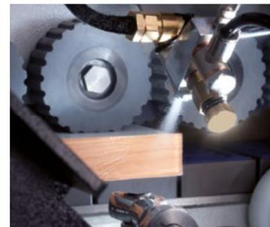
**Spray equipment for the application of solutions to leave a finished work-piece that requires no further processing**
