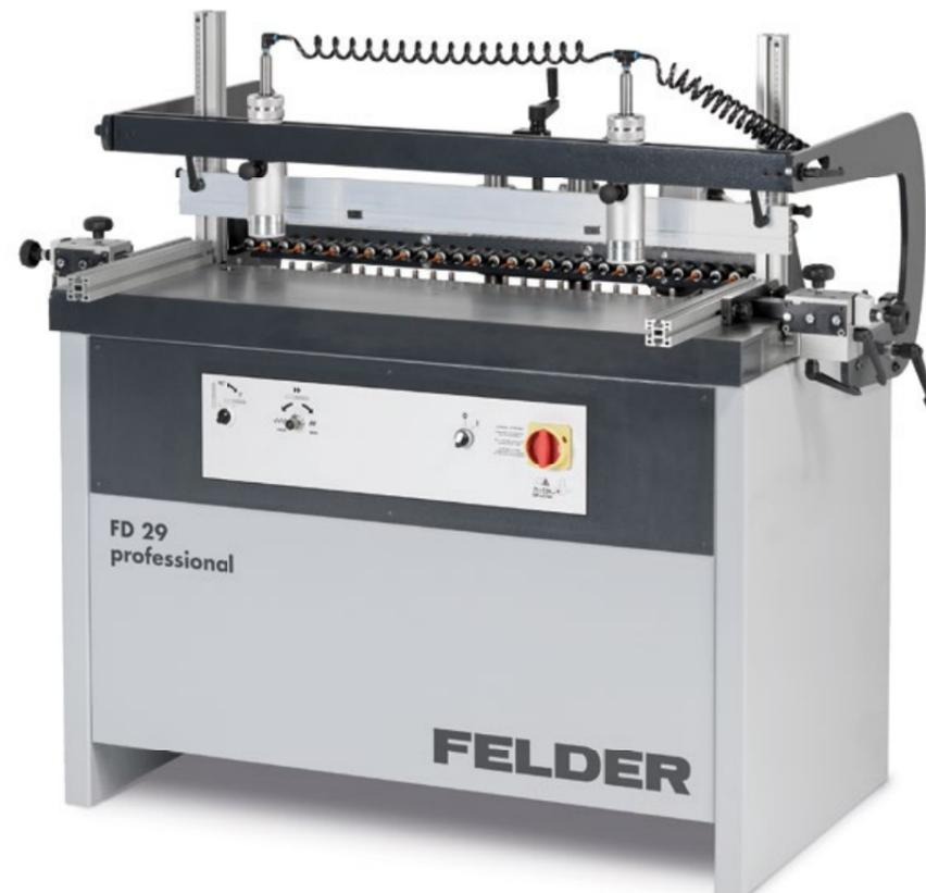
Maximum precision when dowel boring with the Felder FD 29 professional. With 29 high quality drilling spindles at a distance of 32 mm, for drill bits with a diameter of maximum 35 mm, exact dowel and line boring holes are guaranteed. The welded chassis in combination with the solid cast iron table, rigid side and longitudinal stops, as well as pneumatic workpiece holders and ergonomically designed operating elements ensure that the FD 29 professional, is a dowel boring machine of the top class.
