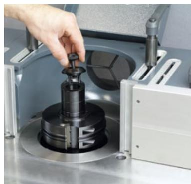
**"Quick-Lock" – change moulding tools quickly and safely**
