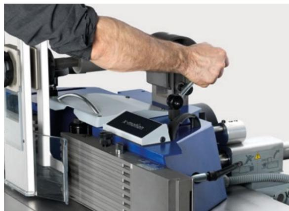
**Spindle moulder fence quick clamping system**
