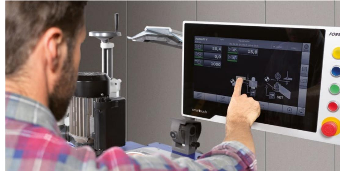
**Spindle fence control via touch screen**
