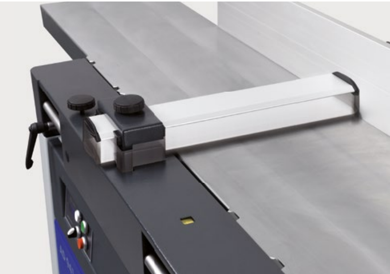
FELDER planer guard Maximum operational safety and maximum user comfort. The space saving planer guard integrated into the machine chassis also stabilises the workpiece when planing and bevelling.
