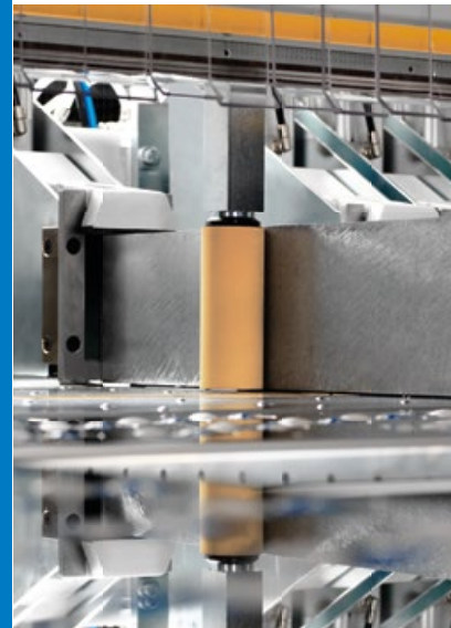
Feeding table with pneumatic pressure roller for exact angular cuts even of long components.
