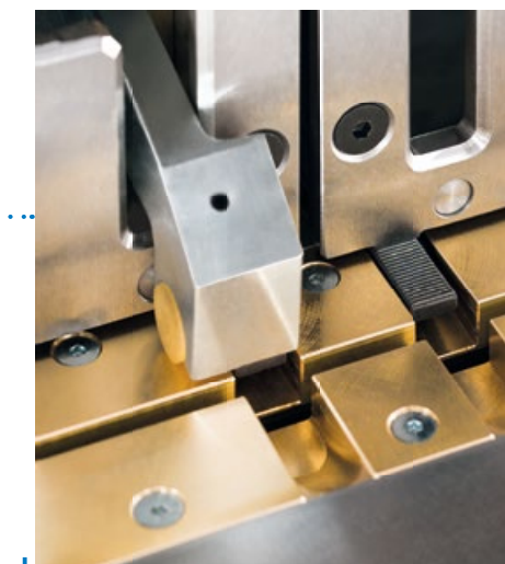
Interchangeable cutting lips made of non-ferrous metal.
