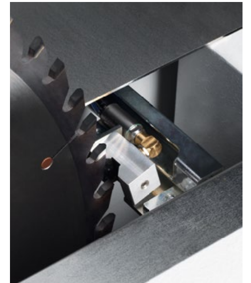
Minimum quantity lubrication system (MMS) integrated in the saw carriage for the main saw blade.
