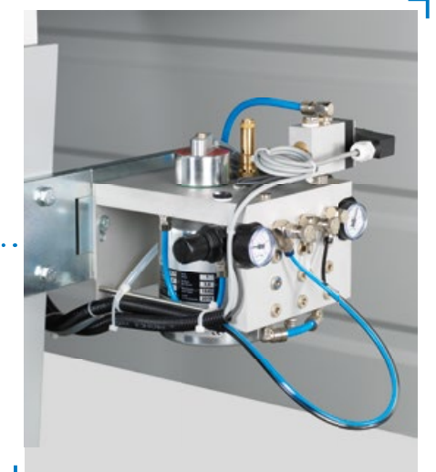
Minimal quantity lubrication system with an ergonomically arranged control unit.
