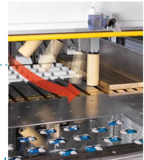
Pneumatically controlled vertical fastening unit for strip cuts.
