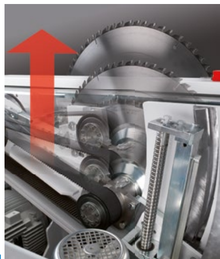
Variable saw blade height adjustment on ground trapezoid guides with backlash-free ball screw.
