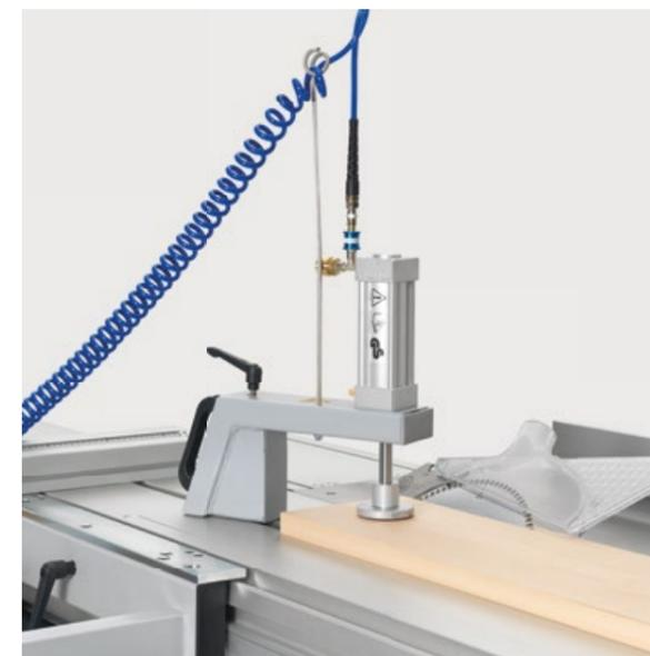
**Pneumatic workpiece holder**
