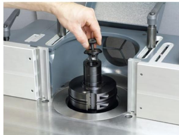
**"Quick-Lock" – change moulding tools quickly and safely**
