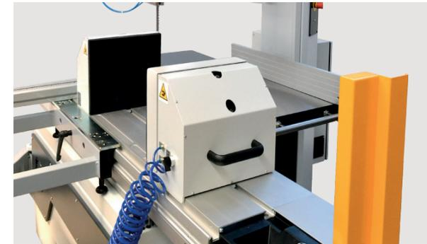
**Clamping system for flat and round components**
